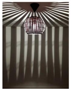
The source is a spherical structure of diameter 29.5cm sectioned at the bottom made of 42 bands of average width 1.26cm opening on 42 slits of average width 0.95cm at mid-height. It can be equipped with a bulb with one or two vertical filaments positioned in its center.
