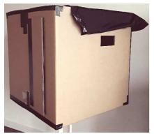
The box used measures approximately 60cmx60cmx60cm. One can also use a box with a little more depth between the slit and the screen and/or a higher height, but it is better to limit the width so that the horizontal movement of the fringes on the screen is observed weak everywhere. On the side, the vertical slit is of high length and in front of it there is a white screen.
