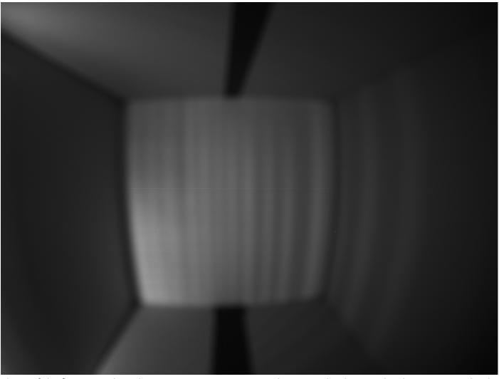
Photo of the fringes made with an astronomy camera. In order to gain brightness, the slit is positioned only 5.50m from the angle of the room. The bulb used is one filament. With two filaments, the fringes have a little more relief and are a little less delimited.
