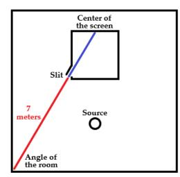
Positioning, not to scale, of the box in top view. The center of the screen, the slit and the angle of the room are aligned. A minimum distance of 6.50m between the slit and the angle must be taken if one wishes a regular image.
