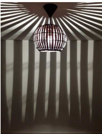
FIG. 1. The source is a spherical structure of diameter 29.5cm sectioned at the bottom made of 42 bands of average width 1.26cm opening on 42 slits of average width 0.95cm at mid-height. It can be equipped with a bulb with one or two vertical filaments positioned in its center.
